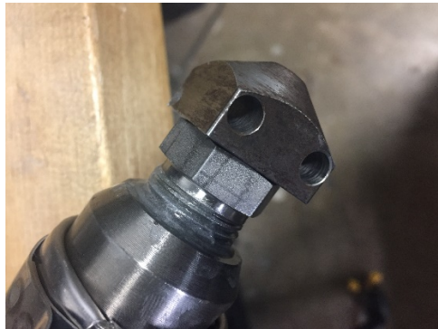
Figure 10 Tip Heater of Small Nozzle for Pellet Extruder. This was included with the Pellet Extruder but was not installed
