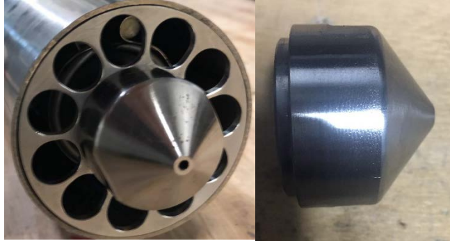
Figure 9 Left: Large Nozzle Screwed onto Extruder Barrel. Right: Large Nozzle Taken off the Extruder Barrel
